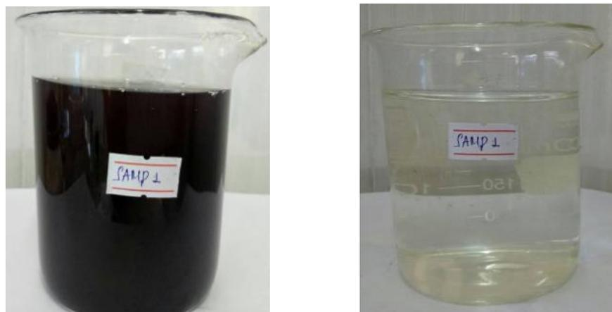
**Fig. 5. Textile dyeing wastewater (left) and catalytic ozonation treatment (right)**
